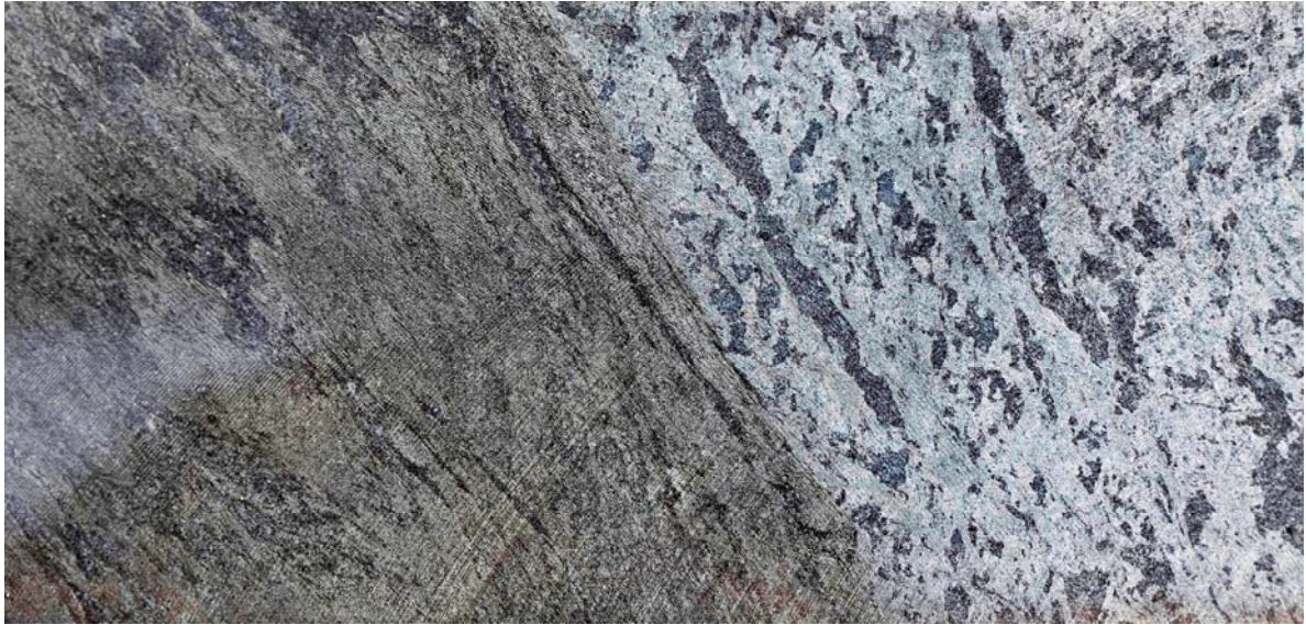
Core photo of KRD10-01 – 30.7 metres - contact of granite (on the right) and chlorite-biotite schist.
