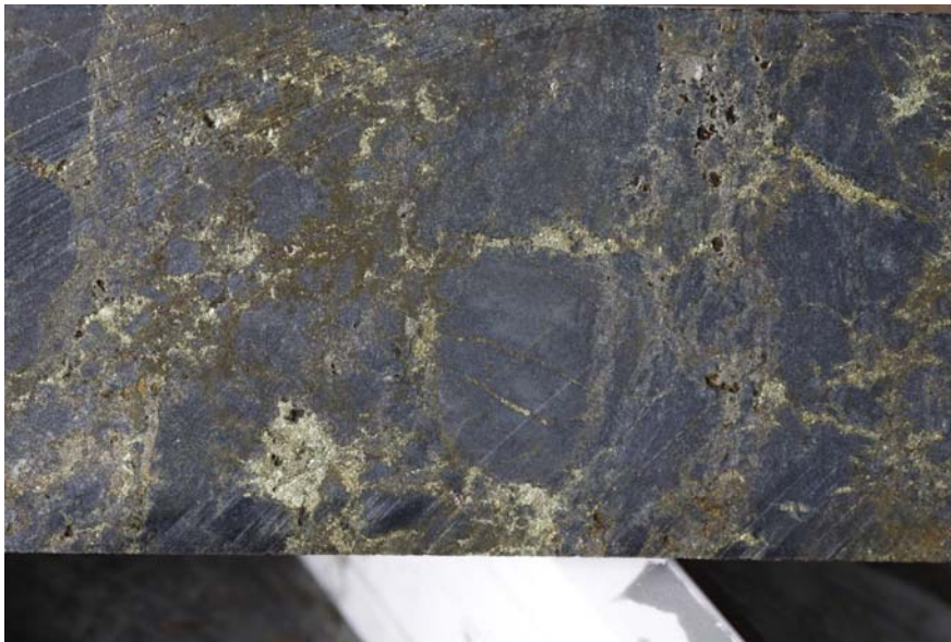
Photo 2 : A Zone Prospect. Chalcopyrite and pyrrhotite in lapilli tuff rocks from drill hole YRC11 - 41D approximately 276 metres down hole. Core approximately 5 cm wide.
